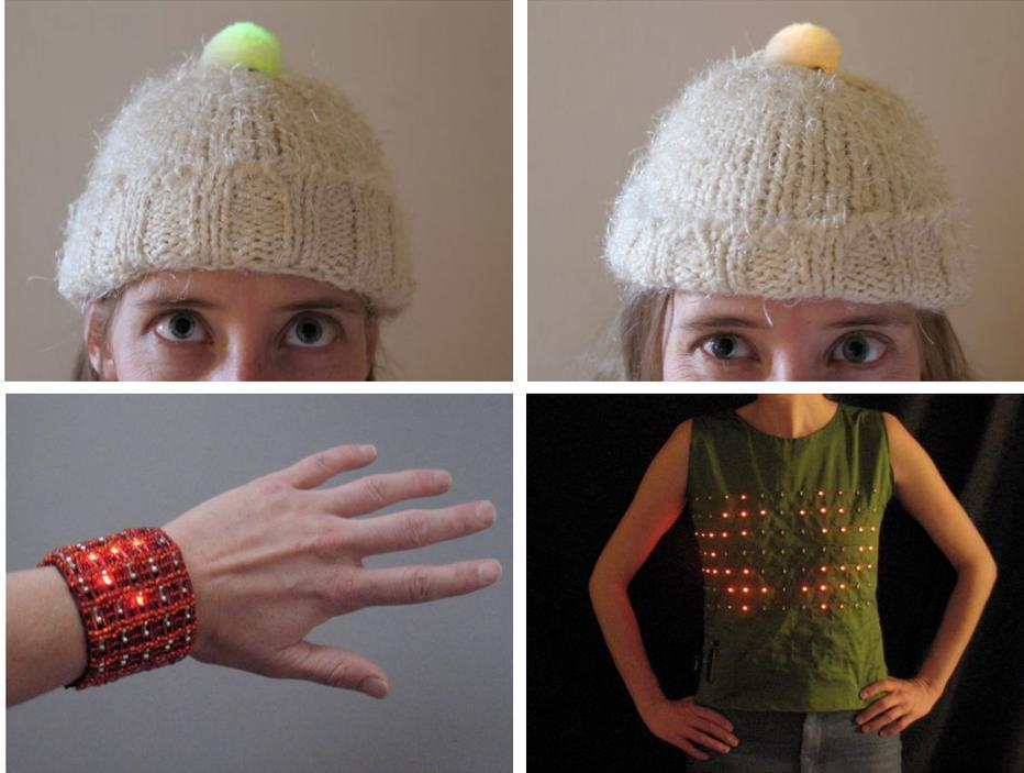
**Figure 6. Top: A temperature-sensing hat. Bottom: Wearable LED displays.**
